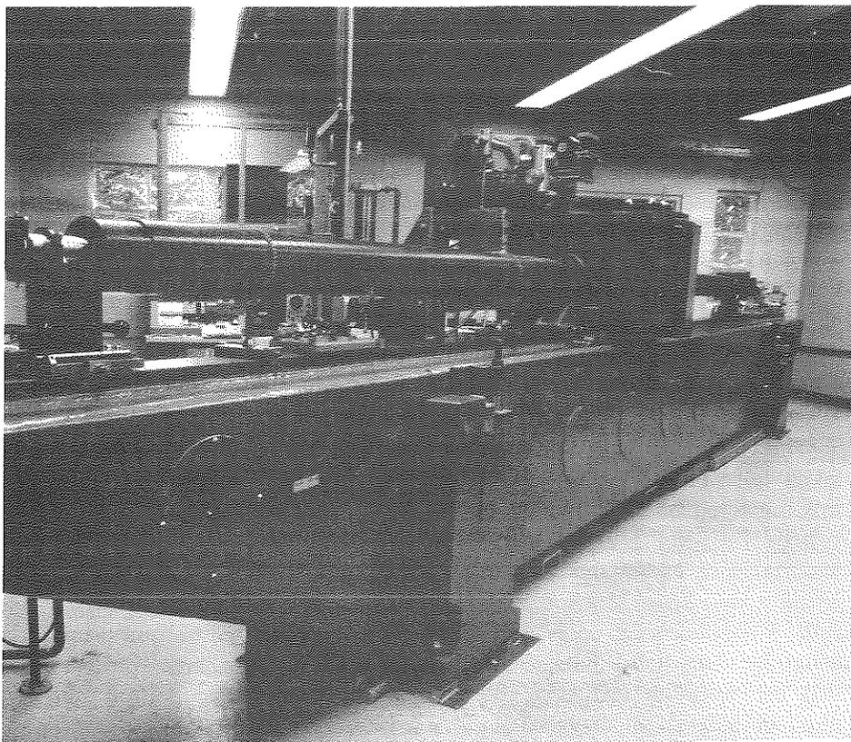
**Fig. 7.** Photograph of the Gosting Diffusimeter at Lawrence Livermore National Laboratory (1986), now at Texas Christian University (Fort Worth, Texas). It can work with both Gouy or Rayleigh optics, and be transferred from one optical system to the other in two minutes.
